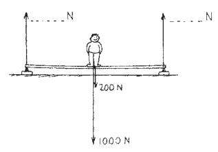
2. When Manuel moves to the left as shown, the scale closest to him reads 850 N. Fill in the weight for the far scale.
