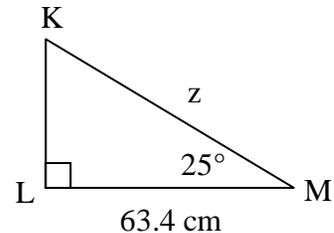
**Step 1:** Place your finger on the acute angle, and then label the three sides: the hypotenuse is always the longest side; the side you are not touching is the opposite leg; and the remaining side you are touching is the adjacent leg.
