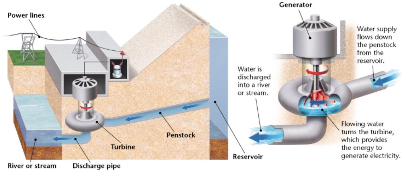
**Figure 9** ► Hydroelectric dams convert the *potential energy*, or stored energy, of a reservoir into the *kinetic energy*, or moving energy, of a spinning turbine. The movement of the turbine is then used to generate electricity.
