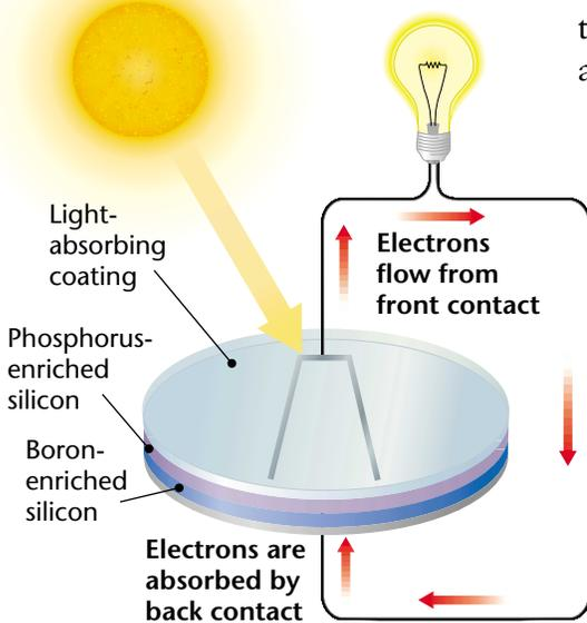
**Figure 5** ▶ Sunlight falls on a semiconductor, causing it to release electrons. The electrons flow through a circuit that is completed when another semiconductor in the solar cell absorbs electrons and passes them on to the first semiconductor.
