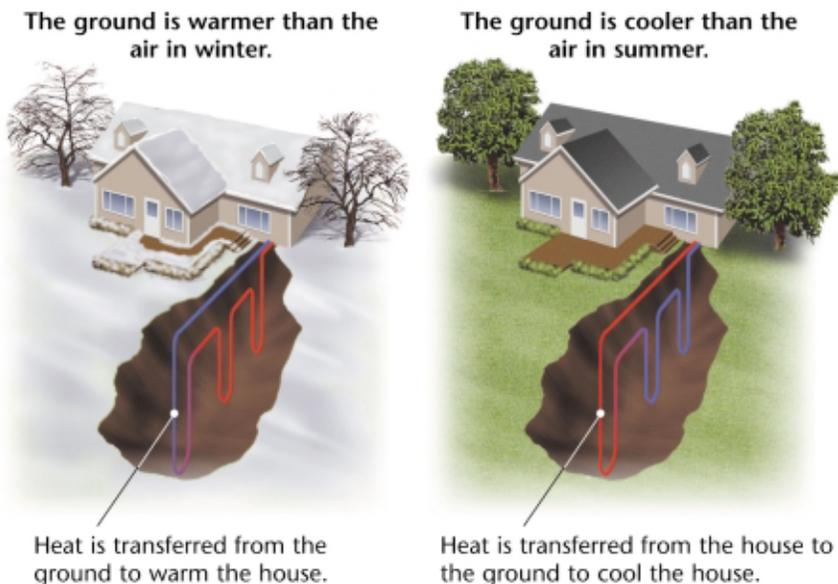
**Figure 12** ▶ In the winter (left), the ground is warmer than the air is. A fluid is circulated underground to warm a house. In the summer (right), the ground is cooler than the air is, and the fluid is used to cool a house.
