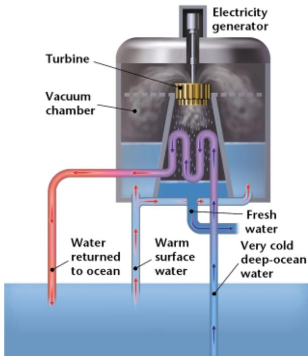
**Figure 14** ► In an open cycle OTEC plant, warm surface water is brought to boil in a vacuum chamber. The boiling water produces steam to drive a turbine that generates electricity. Cold deep-ocean water is pumped in to condense the steam. Fresh water is a byproduct of this type of OTEC plant.
