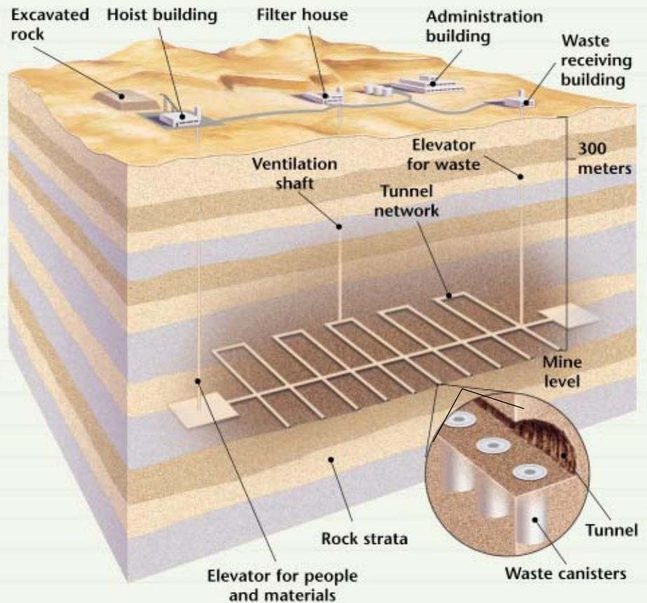
► The preliminary plan for the Yucca Mountain nuclear-waste storage facility shows radioactive materials carefully packaged and buried in tunnels deep underground.
