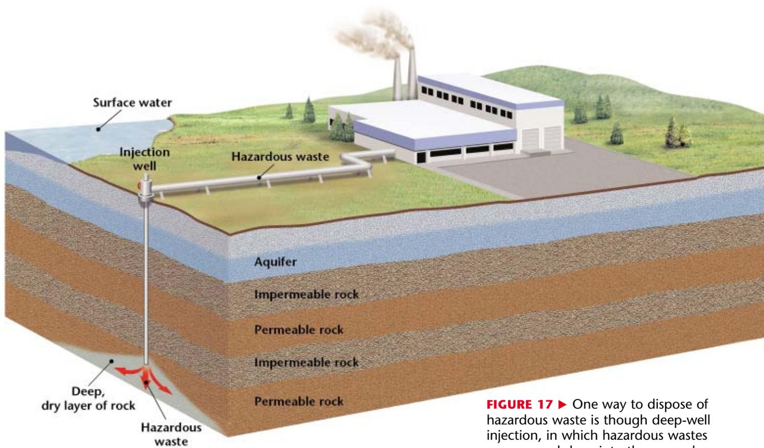
**FIGURE 17** ▶ One way to dispose of hazardous waste is through deep-well injection, in which hazardous wastes are pumped deep into the ground.
