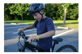
C is for chain. Run the chain by moving the pedals backwards (on a geared bike). Inspect the chain to see that it runs smoothly. If using a geared bike, shift gears to ensure that the entire mechanism (drive train) runs smoothly.
